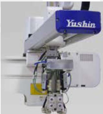
Fig 1: Full Servo Robot / 32 Cavity End of Arm Tool (EOAT)
