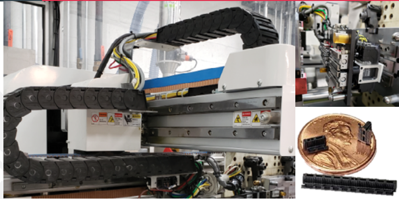
Fig 1: High Speed 2 Axis Side Entry Robot with Part Inspection Capabilities
